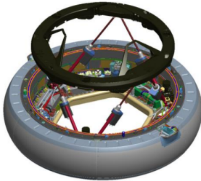
Figure 9: NASA Docking System
